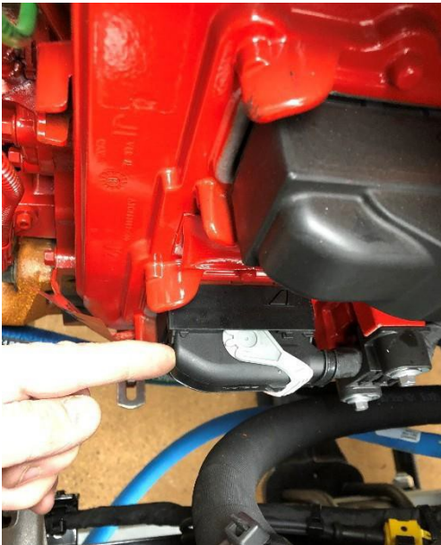
Figure 25 Cummins ECM J2 Connector
