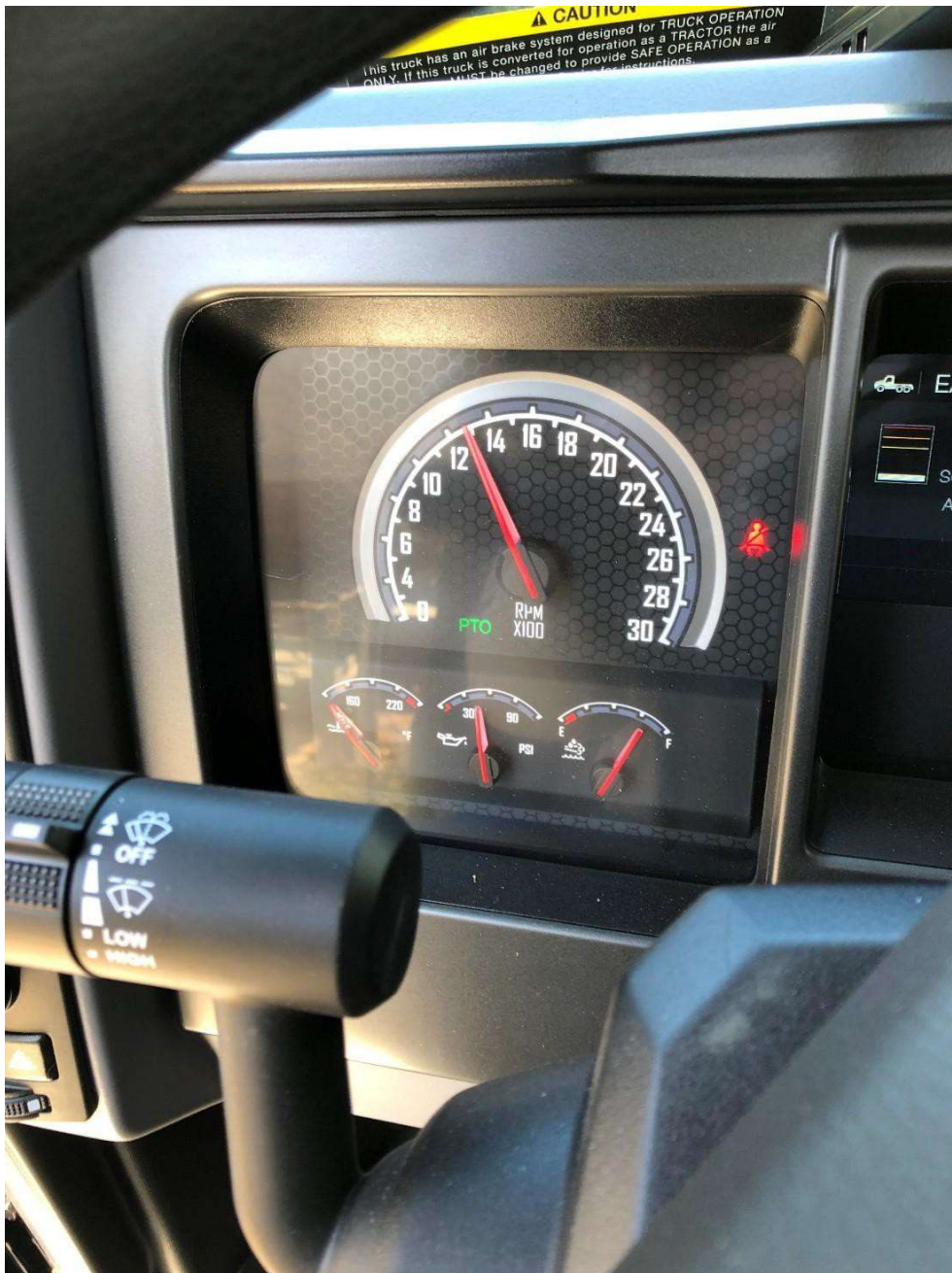
Figure 24 PTO Icon Illuminated in Tachometer
